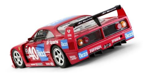
The body, designed by Pininfarina, Nicola Materazzi e Pietro Camardella, was made of carbon fiber and composite materials, and had a weight of 46 kg. The F40 had a maximum speed of 326 km/h.
